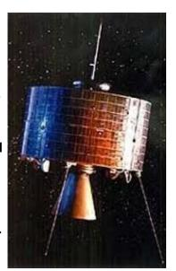
tions carried by satellites. It could handle one telephone conversation or up to fifteen teletype communications.
